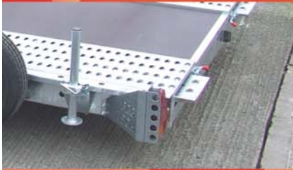
WELL PROTECTED LIGHTING SYSTEM AND REAR SUPPORT STANDS
