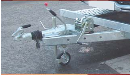
BRADLEY CAST BODY / HEAD HITCH AND TWO SPEED WINCH
